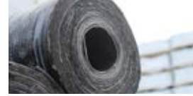
SBS roofing material
