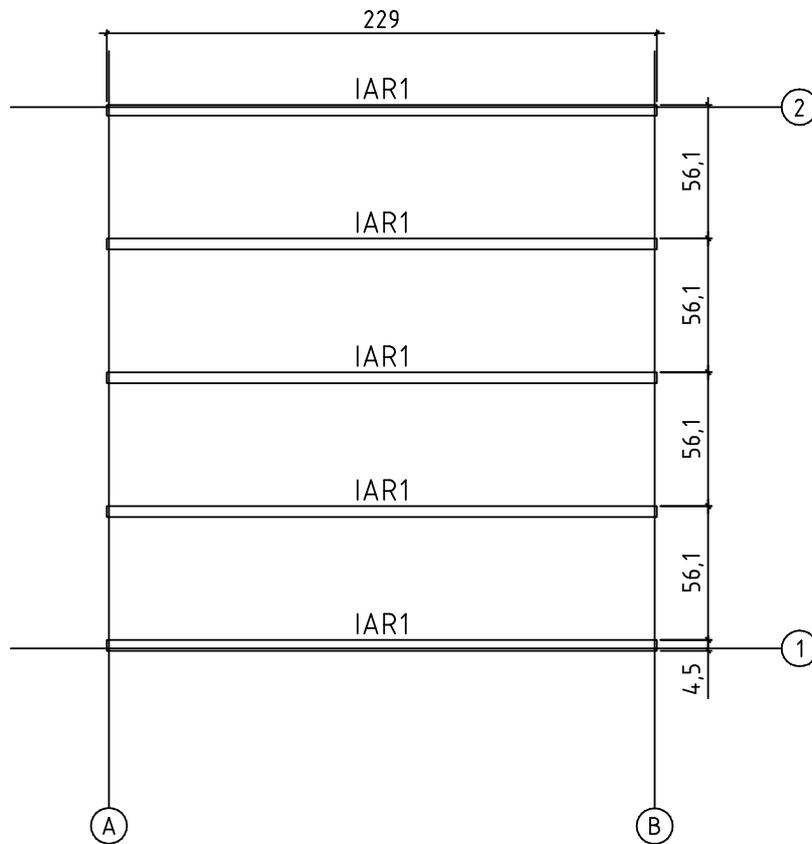
FLOOR BOARDS - FUSSBODENBRETTER - PLAN POSE PLANCHER
